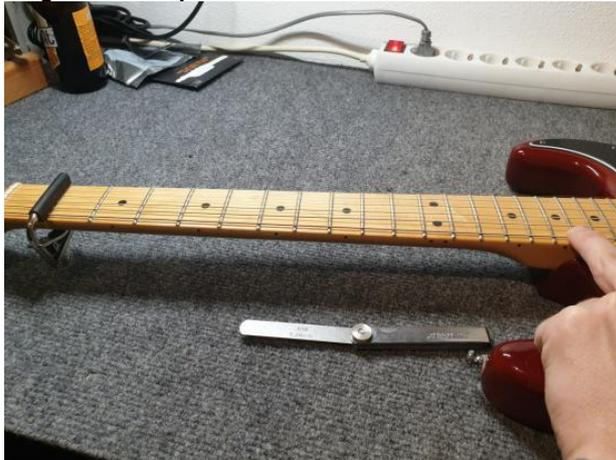
Now you have to use a feeler gauge. For a normal and good setup like this you should use 0.25mm/.010 and measure the distance between the 8<sup>th</sup> fret and the string (measure the High E and Low e string). The gap should be the same thickness as the feeler gauge.
